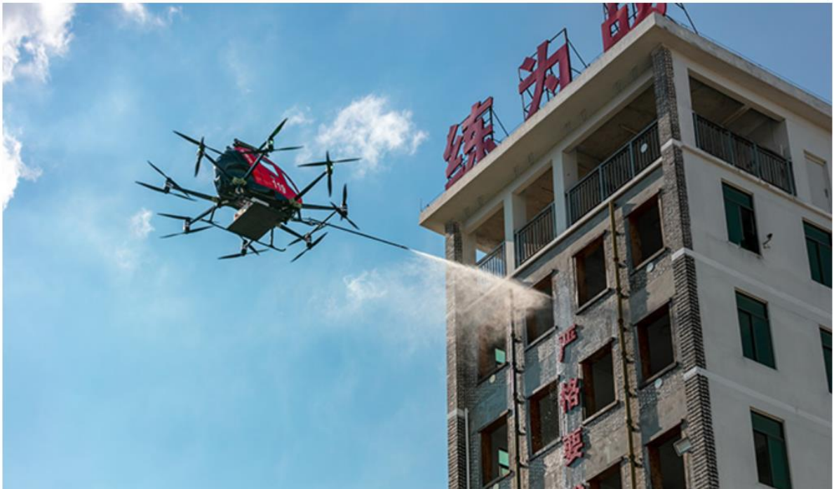
Figure 15: EHang 216F Extinguishing Fire
